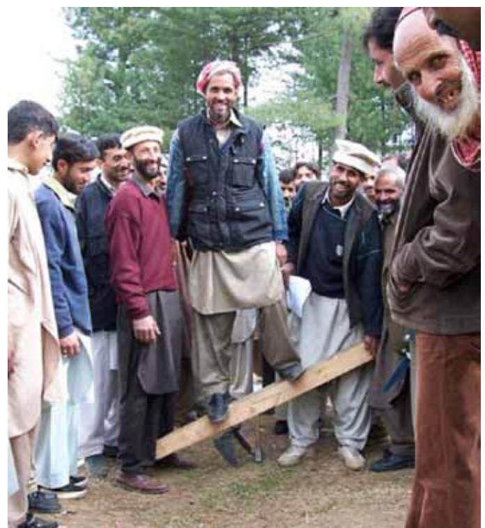
b) Testing strength of a timber joint (source: Kubilay Hicyilmaz).
